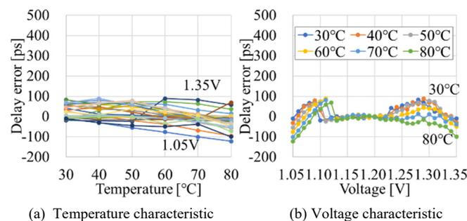
Figure 9. Evaluation of correction using polynomial approximation.
