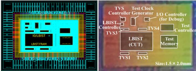
(a) Chip layout (b) Fabricated test chip
