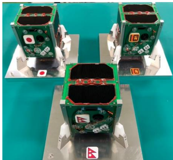
Figure 21. Flight Model CubeSats of BIRDS-3. CubeSat at the left top most corner is the Uguisu which carries SoftCIB.
