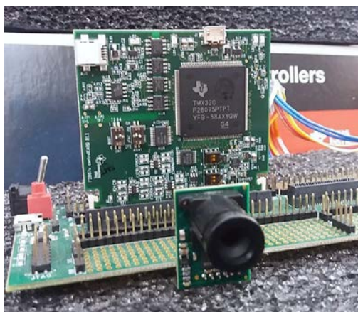
Figure 15 Camera selected for the AV4 mission and development board
