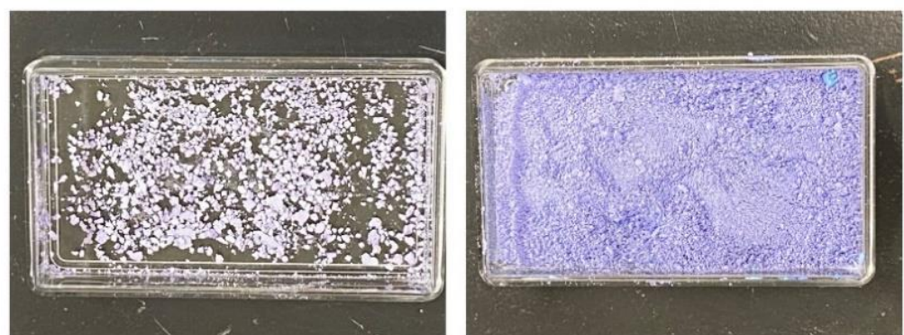
Figure 6. Appearance of OCP microspheres after immersion in the methylene blue solution (Left) and microspheres prepared with the addition of methylene blue (Right).
