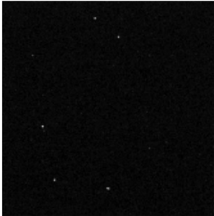
Fig. 2. Example of actual star image from star sensor
