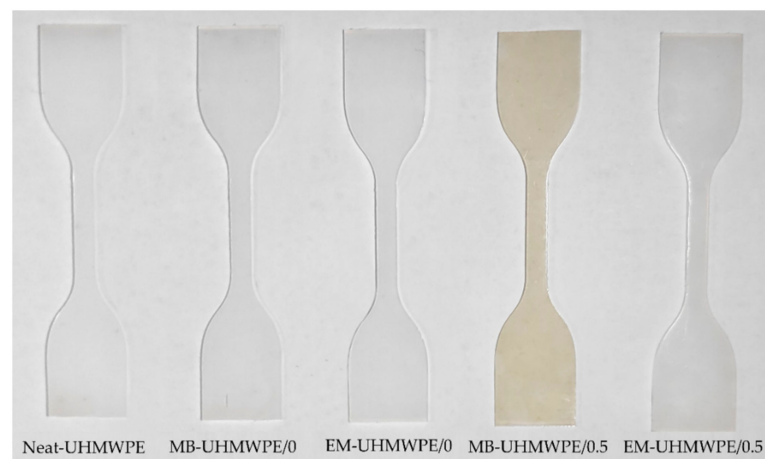
Figure 5. The visual appearance of polymer and UHMWPE/CNF bionanocomposites samples produced through melt blending and ethanol mixing.
