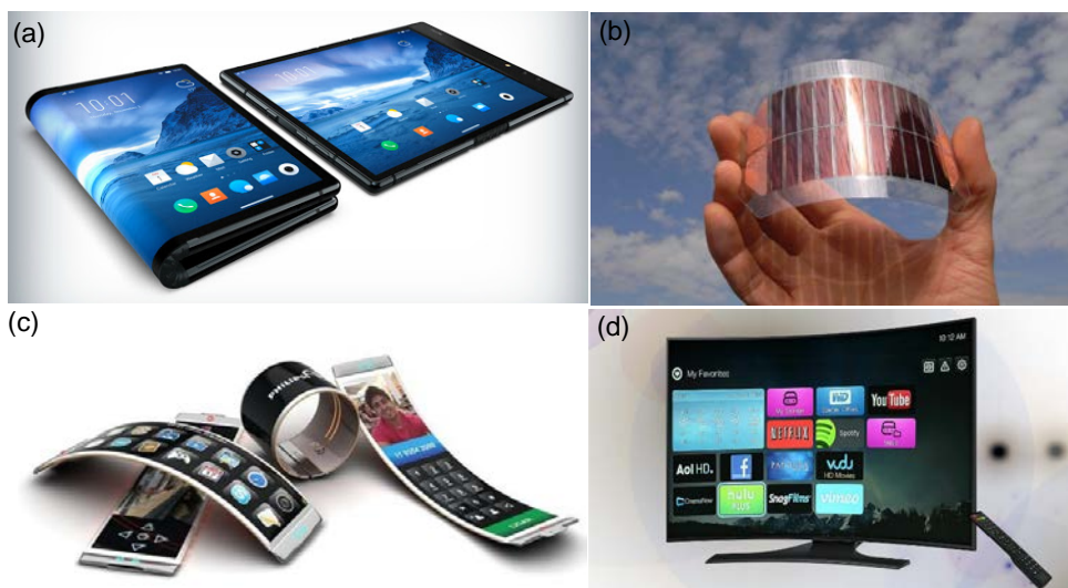
Figure 1.2 Digital image of some organic electronic devices (a) the foldable FlexPai smartphone/tablet 7 ; (b) flexible organic solar cell 8 ; (c) wearable smartphones 9 ; (d) Flexible TV (source: FlexEnable) 10 .
