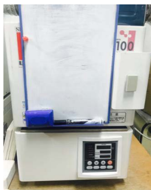
Figure-11. Photograph of the muffle furnace used to prepare \text{TiO}_2 coated FTO glass substrate.
