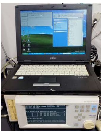
Figure-9. An auto-polarization system (HSV-100) used for the CV measurement in this work.
