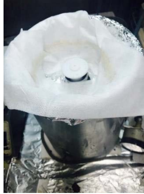
Figure-13. Spin coater for preparing counter electrode.
