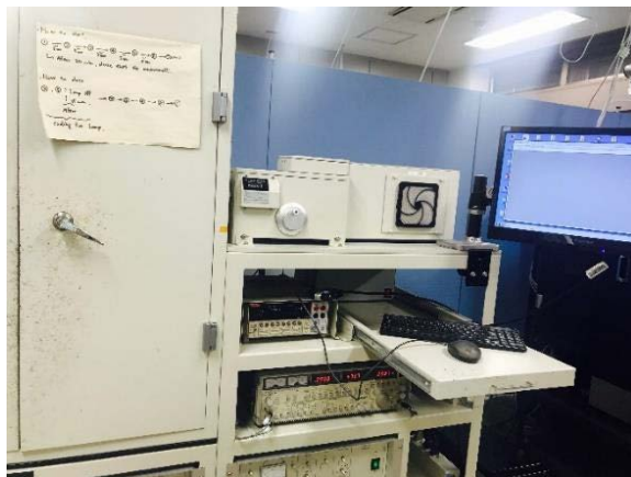
Figure-15. Photograph of the solar simulator utilized for photovoltaic characterization of the DSSCs fabricated in my research.
