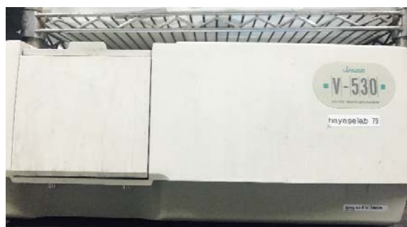
Figure -3. UV-Visible spectrophotometer used for measuring the electronic absorption spectra.
