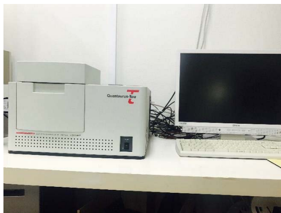
Figure-4. Fluorescence and fluorescence lifetime measurement system.
