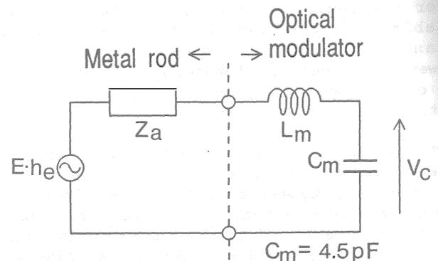
Fig.3 Equivalent circuit of the sensor.
