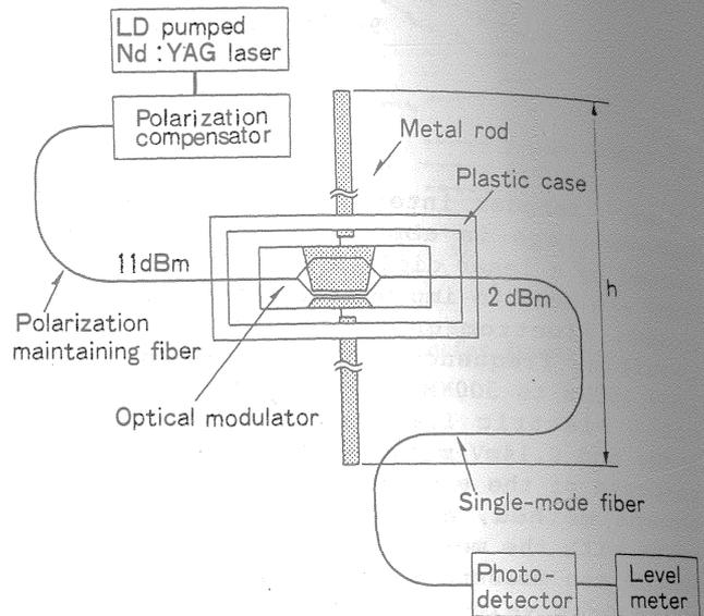
Fig.1 Configuration of electric field sensor.
