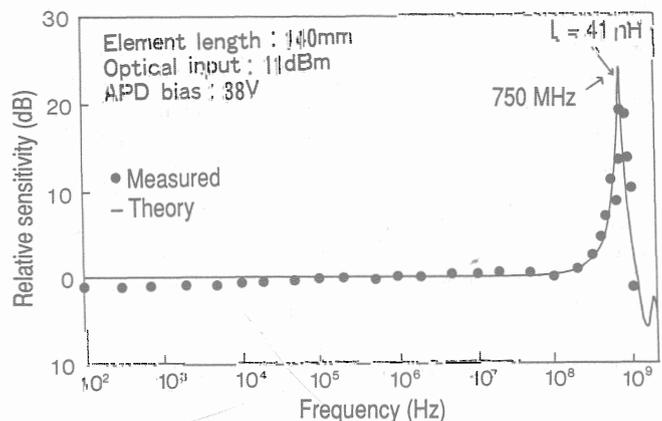
Fig.5 Frequency response of the sensor.
