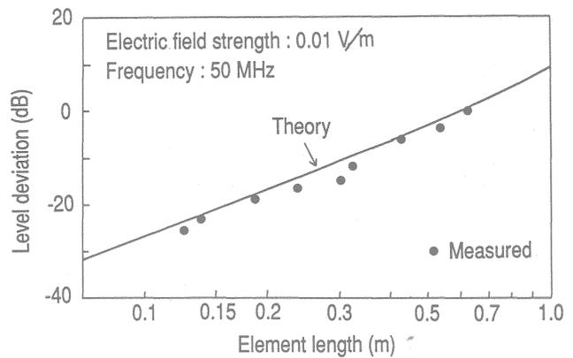
Fig.10 Dipole element length dependence of the sensor.
