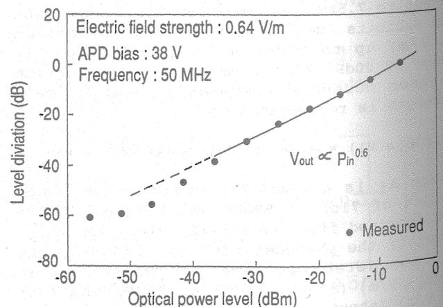
Fig.8 Optical power dependence of the sensor.
