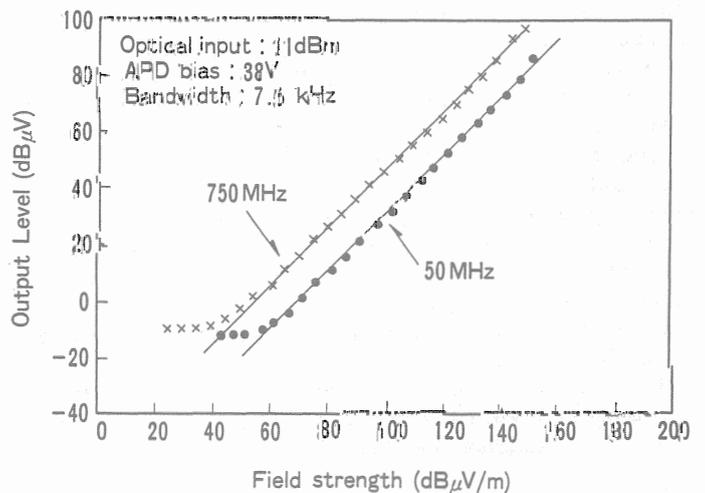
Fig.6 Sensitivity of the sensor.
