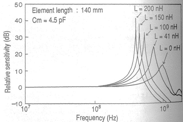
Fig.7 Calculated frequency response of the sensor.
