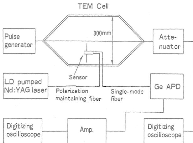
Fig.12 Experimental setup for measuring impulse response of the sensor.
