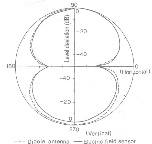
Fig.11 Cross-polarization of the sensor.
