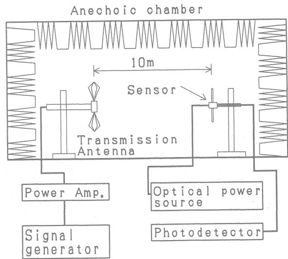
Fig.9 Experimental setup for measuring dipole element length dependence and cross-polarization.
