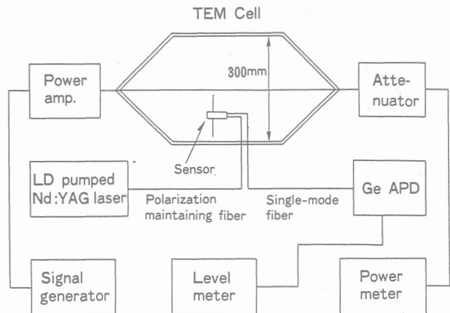
Fig.4 Experimental setup for measuring sensitivity of the sensor.
