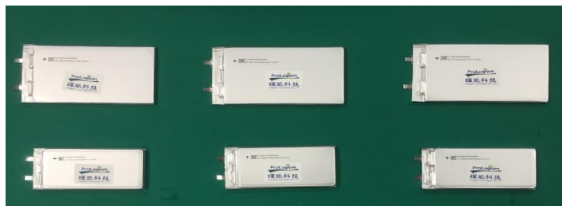
Fig IV-1 SSLCBs group selected for the launch environment ground evaluation test [24]
