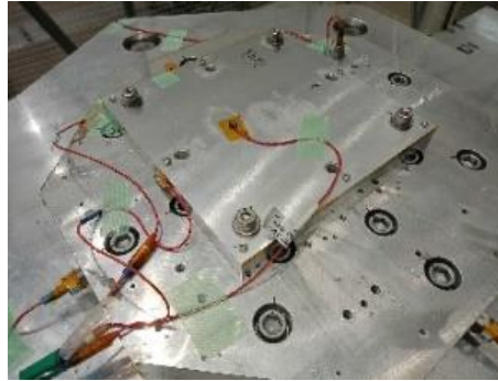
Fig IV-5 The shock test’s jig with pickup sensors configuration [24]
