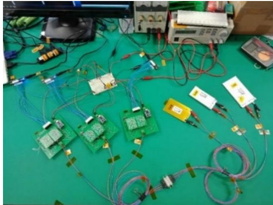
Fig IV-18 Testing the test board with Solid-State-Ceramic battery The same setup used during the charge and discharge before and after each test [13]
