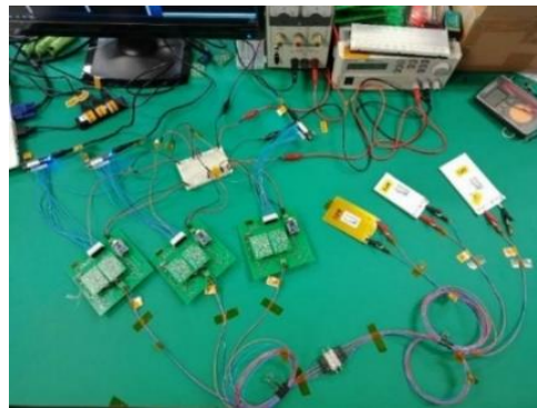
Fig IV-2 Solid-State-Ceramic battery functional test Charged and discharged before and after each test [24].
