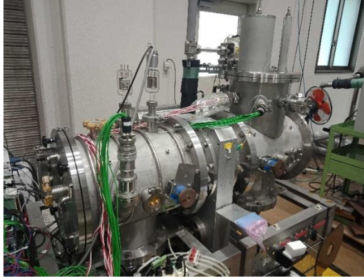
Fig IV-10 Thermal Vacuum Chamber (TVAC) The Kyushu Institute of Technology LaSEINE laboratory [13,96]
