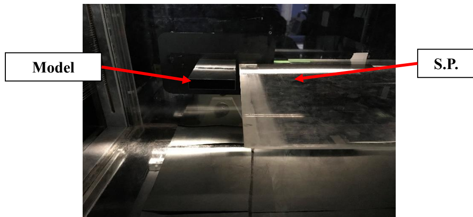
Figure 4.1.6 Setting situation of the S.P. inside the wind tunnel
