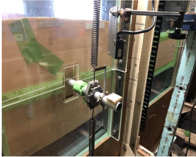
Figure 6.1.8 Suspension situation outside the wind tunnel
