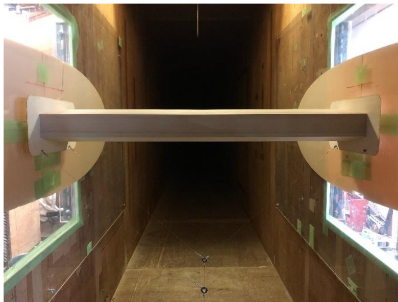
Figure 6.1.5 Sectional model of TYPE-1 cross section ( \theta=10^\circ ) inside the wind tunnel
