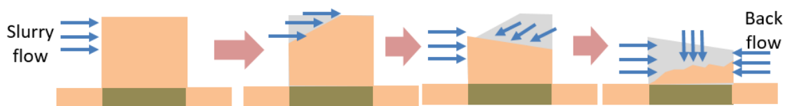
Fig. 6 Progress of material decreasing as Slurry flow field continue during CMP.
