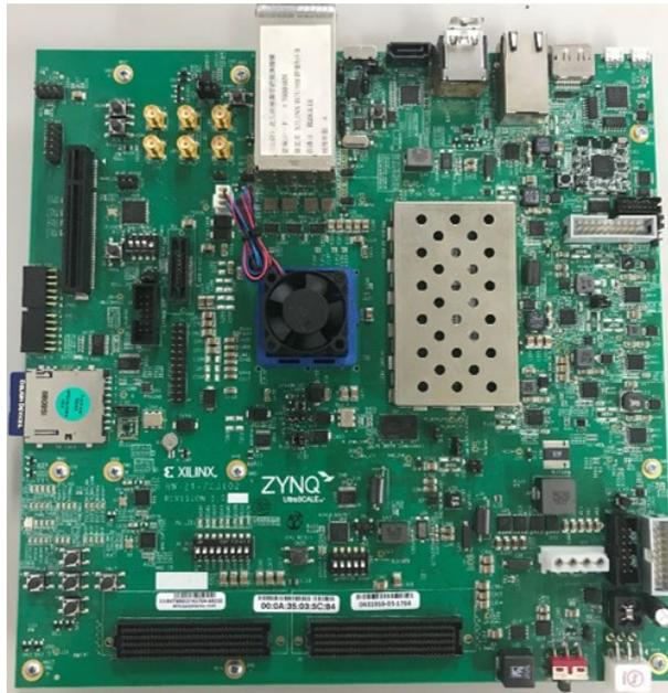
**Fig 2.8.** A image of a FPGA board, Zynq UltraScale+ MPSoC ZCU102 Evaluation Kit
