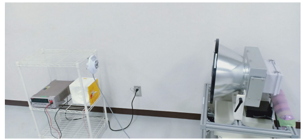
Fig. 22. Test setup using sun simulator, sourcemeter and pyranometer as irradiance reference.
