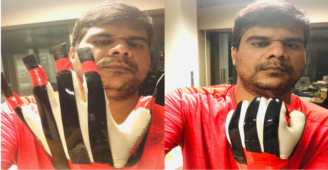
Fig. 4: LEAP technology's sensor fixed on stretchable glove for taking data for hand gesture recognition in open and fist position of hand
