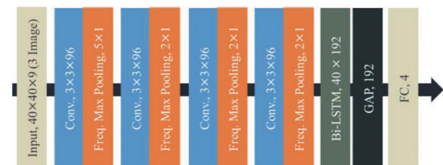
Fig.3 Architecture of improved CRNN Freq. Max Pooling : Frequency Max Pooling, GAP : Global Average Pooling
