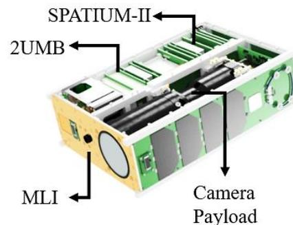
Fig. 4. KITSUNE configuration with 2UMB, SPATIUM-II and 3U camera payload in addition to the MLI on nadir pointing side.
