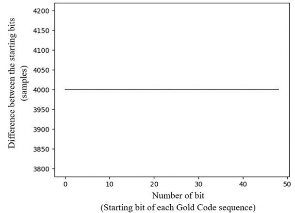
Fig. 9: Cross correlation results showing the difference between the gold code sequence starts.
