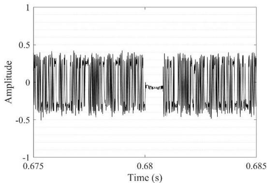
Fig. 8. RF switch detection onboard during the ground tests at 0.68 s.
