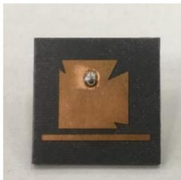
Fig. 5. 5.8 GHz C-band patch antenna.
