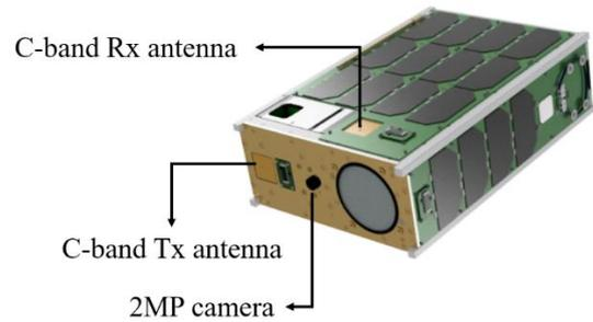
Fig. 6. C-band antennas and 2MP camera.
