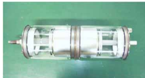
b) Prototype vacuum interrupter used in the vacuum circuit breaker
